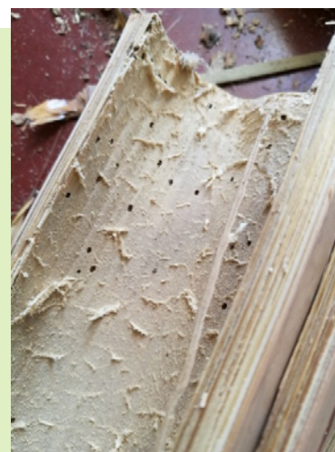
Figure 8. Defective bamboo logs with cracks, ruptures and splits, and irregular shapes. These defects are were probably due to excessively high temperatures or sudden temperature fluctuations, which caused irregular drying during the six-month drying process © Chuen Mun Wai
