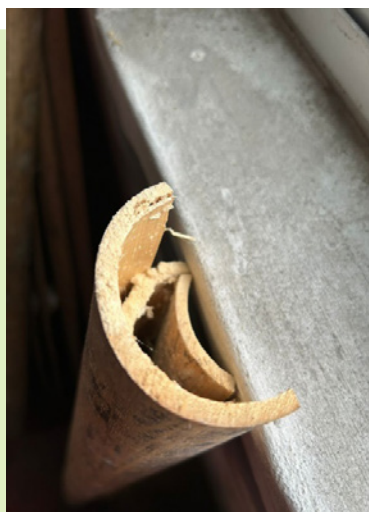
Figure 8. Defective bamboo logs with cracks, ruptures and splits, and irregular shapes. These defects are were probably due to excessively high temperatures or sudden temperature fluctuations, which caused irregular drying during the six-month drying process © Chuen Mun Wai
