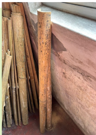
Figure 8. Defective bamboo logs with cracks, ruptures and splits, and irregular shapes. These defects are were probably due to excessively high temperatures or sudden temperature fluctuations, which caused irregular drying during the six-month drying process © Chuen Mun Wai
