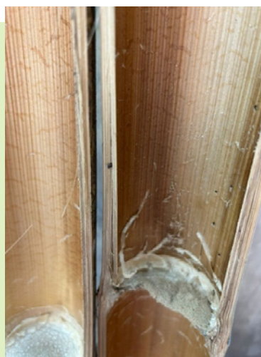
Figure 9. Defective bamboo logs with small holes, a result of infestation by ants, spiders and scorpions © Chuen Mun Wai
