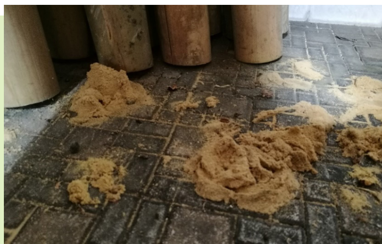
Figure 10. Defective bamboo logs with powdery dust from bamboo holes after insect infestation © Chuen Mun Wai
