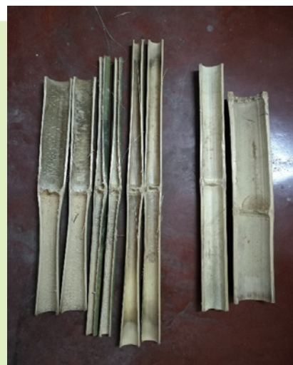
Figure 8. Defective bamboo logs with cracks, ruptures and splits, and irregular shapes. These defects are were probably due to excessively high temperatures or sudden temperature fluctuations, which caused irregular drying during the six-month drying process © Chuen Mun Wai
