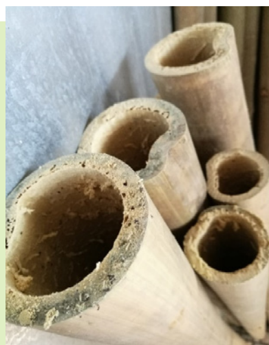
Figure 9. Defective bamboo logs with small holes, a result of infestation by ants, spiders and scorpions © Chuen Mun Wai
