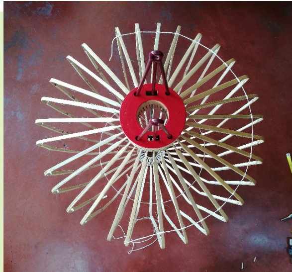
Figure 5. Crafting process: Traditional thread-tying technique to strengthen the shape of the assembled frame structure © Chuen Mun Wai
